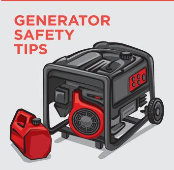
N ever connect a standby generator into your home's electrical system. There are only two safe ways to connect a standby generator to your equipment.
